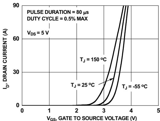
Figure 5. Transfer Characteristics
