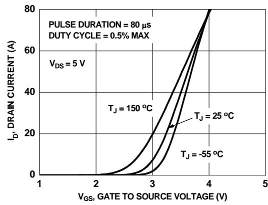
Figure 5. Transfer Characteristics
