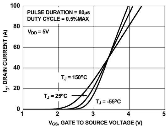
**Figure 5. Transfer Characteristics**
