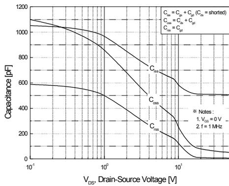
Figure 5. Capacitance Characteristics
