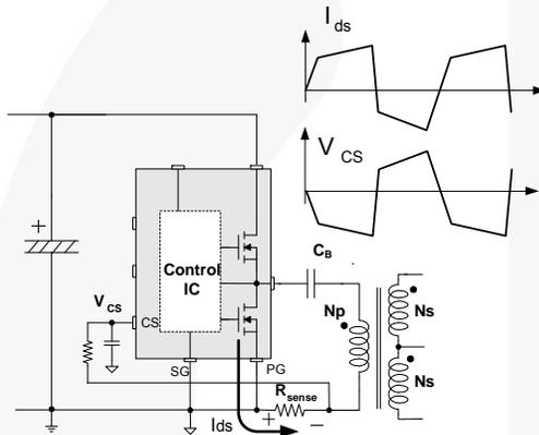
**Figure 22. Full-Wave Sensing**
