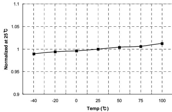
Figure 16. V<sub>LIM</sub> Voltage vs. Temperature
