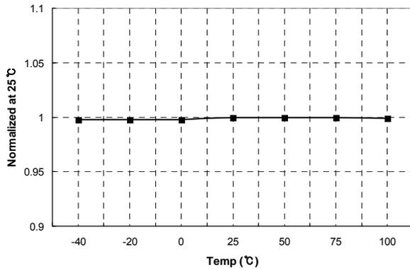
Figure 7. High-Side  $V_{CC}$  ( $HV_{CC}$ ) Start vs. Temperature
