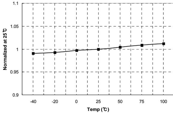
Figure 13. LV<sub>CC</sub> OVP Voltage vs. Temperature
