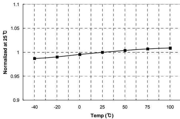
Figure 15. V<sub>BH</sub> Voltage vs. Temperature
