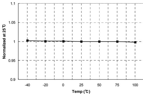
Figure 9. Low-Side  $V_{CC}$  ( $LV_{CC}$ ) Start vs. Temperature
