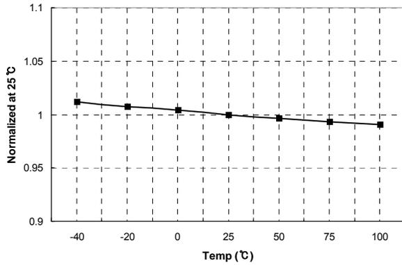
Figure 5. Maximum Duty Cycle vs. Temperature
