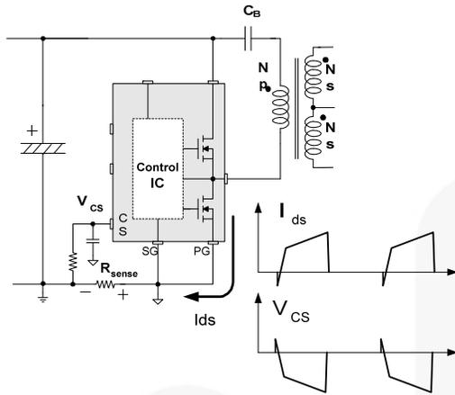
**Figure 21. Half-Wave Sensing**
