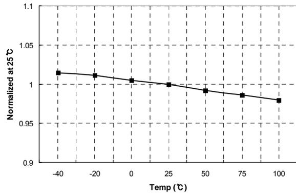
Figure 8. High-Side  $V_{CC}$  ( $HV_{CC}$ ) Stop vs. Temperature
