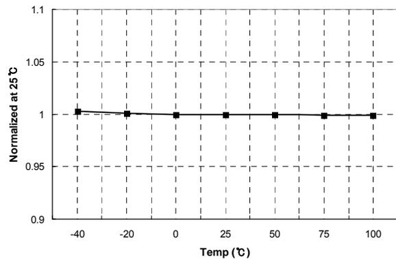
Figure 10. Low-Side  $V_{CC}$  ( $LV_{CC}$ ) Stop vs. Temperature
