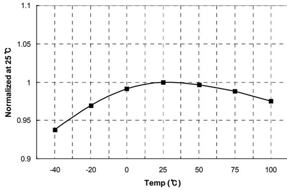
Figure 11. OLP Delay Current vs. Temperature
