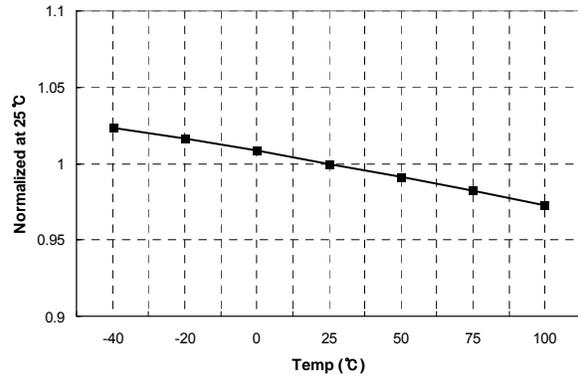
Figure 6. Switching Frequency vs. Temperature
