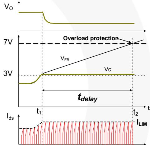
**Figure 23. Overload Protection**
