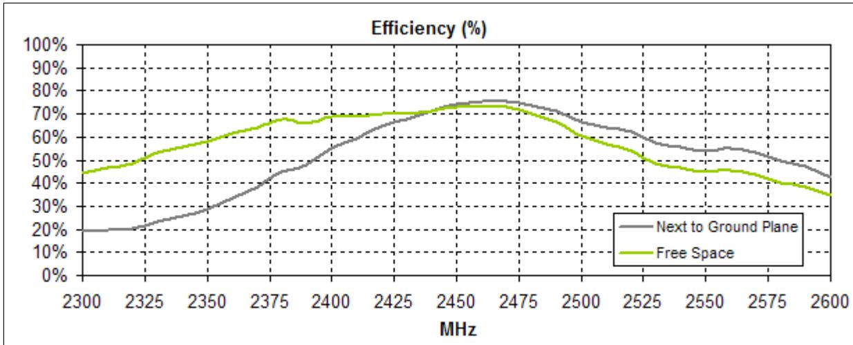
Figure 7. Efficiency for the FXP72 Antenna.
