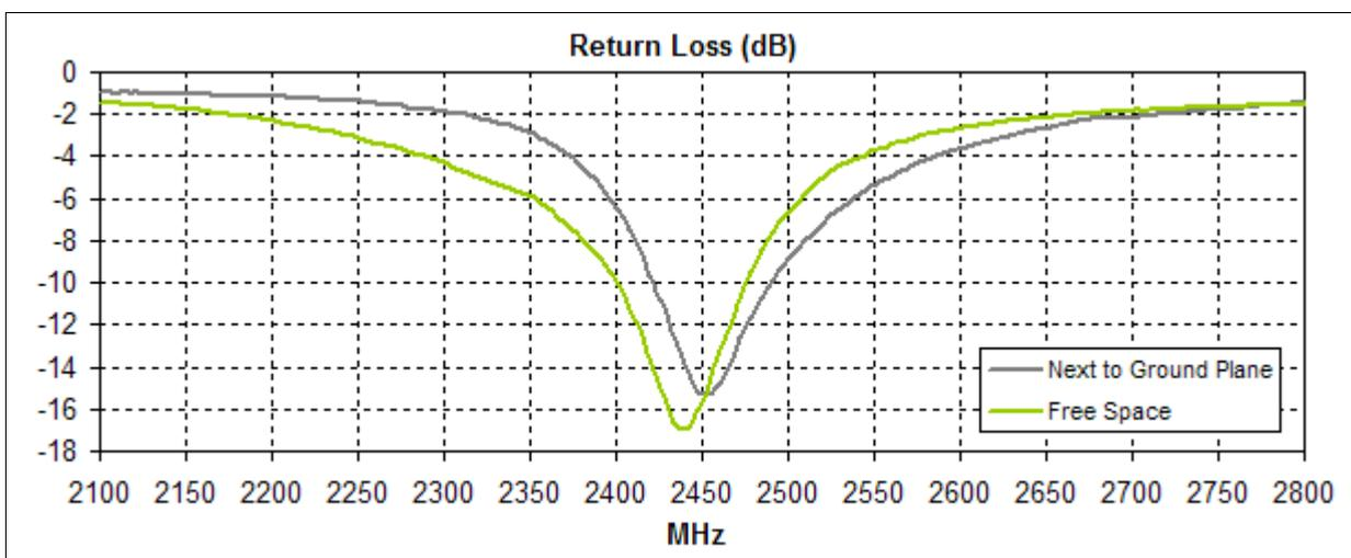
**Figure 3.** Return Loss for the FXP72 Antenna.
