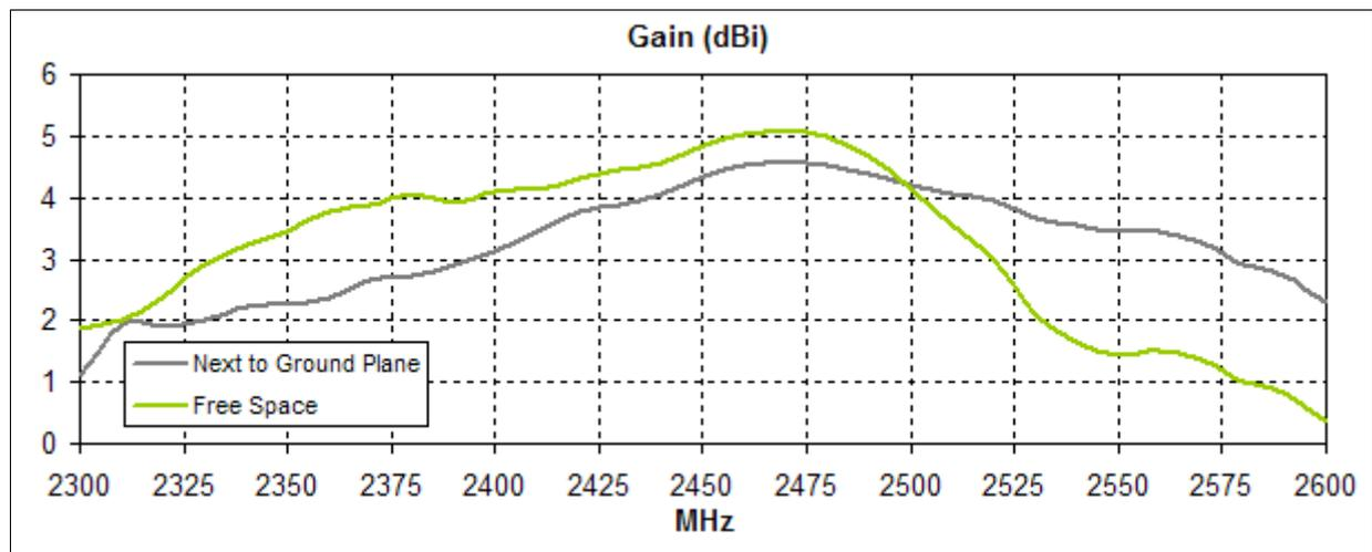
**Figure 6.** Gain for the FXP72 Antenna.
