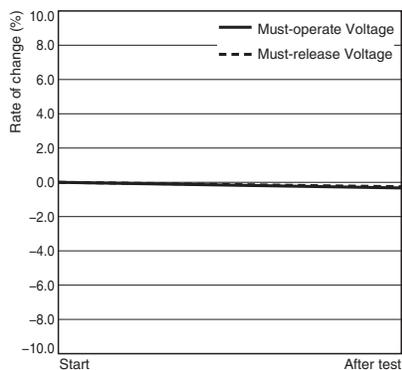
Characteristics were measured after applying a shock of 490 m/s<sup>2</sup> to the test piece 3 times each in 6 directions along 3 axes. The percentage rate of change is the average value for all of the samples.
