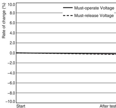
Characteristics were measured after applying vibration at a frequency of 5 to 200 to 5Hz, acceleration of 44.1 m/s<sup>2</sup> to the test piece (not energized) for 2 hours each in 3 directions. The percentage rate of change is the average value for all of the samples.
