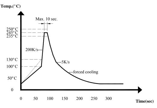
Recommendable wave soldering condition is as follows. Note 1: It is requested that wave soldering should be executed after heat of product goes down to normal temperature.
