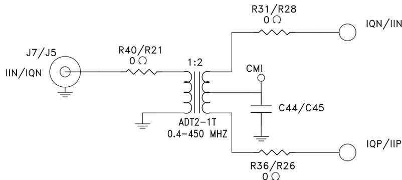
Figure 4. HMC960LP4E Evaluation Board Single-Ended Input Configuration
