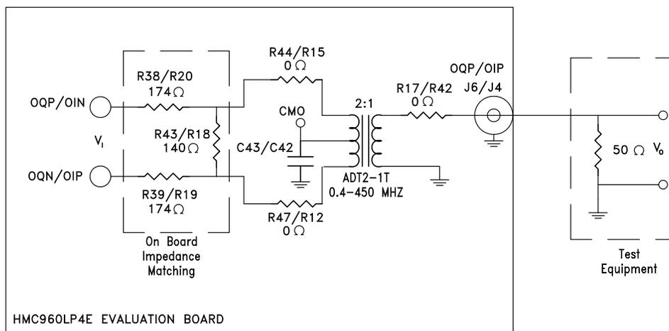
Figure 5. HMC960LP4E Evaluation Board Single-Ended Output Configuration
