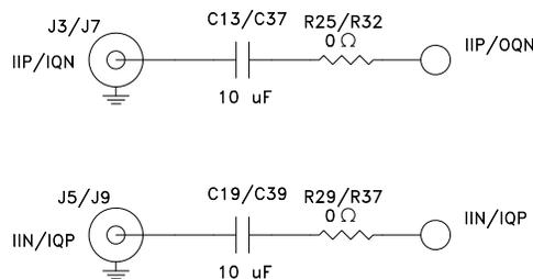
Figure 2. HMC960LP4E Evaluation Board Default Differential Input Configuration
