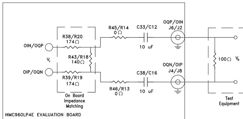
Figure 3. HMC960LP4E Evaluation Board Default Differential Output Configuration
