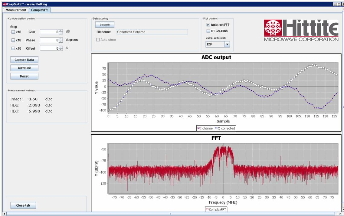
Figure 45. EasySuite result showing not changing the DCR configuration but changing the input signal to 4 carrier WCDMA (Filter bandwidth setting is 5 MHz)
