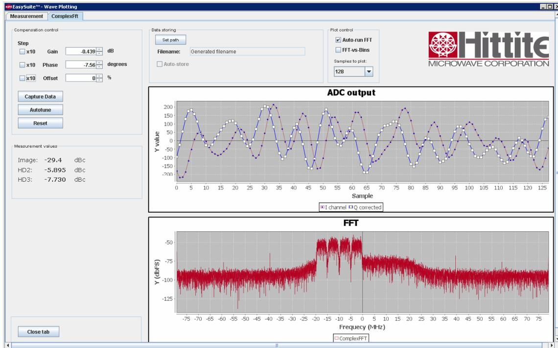
Figure 51.DCR EasySuite showing received four carrier WCDMA signal after executing calibration algorithm. The image is eliminated and calculated amplitude and phase miss match is virtually identical to those calculated using single-carrier WCDMA signal earlier.
