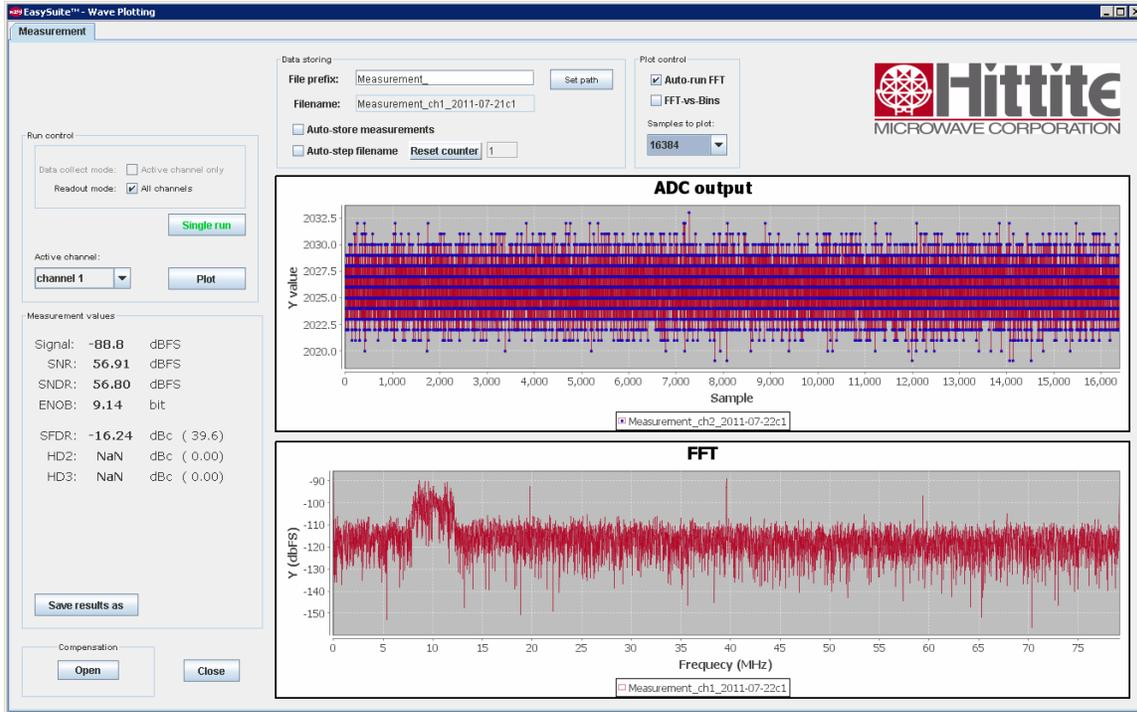
Figure 21. EasySuite Measurement View
