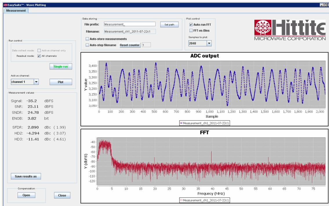
Figure 35. Observed results when second VGA gain increased by 5 dB with filter bandwidth set to 5 MHz
