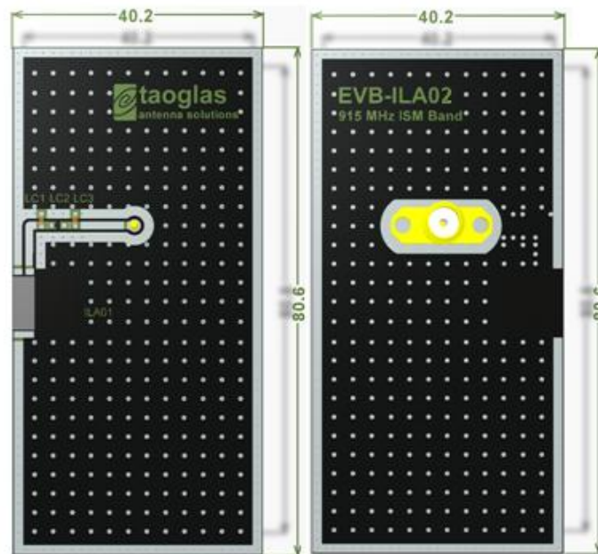
Figure 9. Test evaluation board with antenna. Top layer (left hand) and Bottom layer (right hand)
