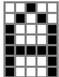
the character graphic and the 7th byte is the bottom row of the character graphic. The B7 of each byte of the character graphic data is the leftmost column of the character graphic. B2, B1 and B0 are not used and should be set to zero.
