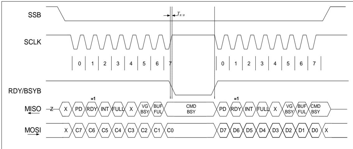
Figure 8-2 RDY/BSYB Timing for SPI Writing Transactions.
