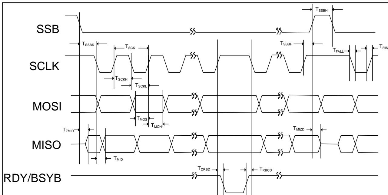
Figure 12-1 SPI Timing
