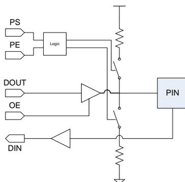
Figure 6-1 GPIO Structure
