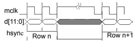
Figure 20:  $hsync$  Timing
