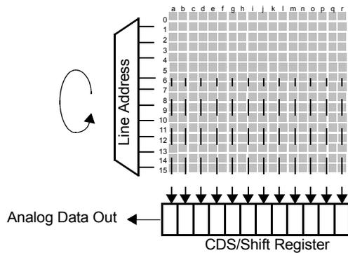
Figure 7: CMOS APS Row and Column addressing scheme
