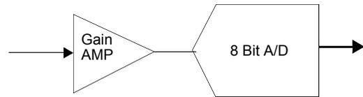
Figure 8: Analog Signals In, Digital Data Out.
