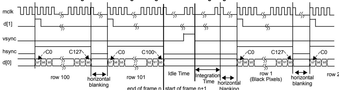
Figure 27: Serial Digital Image Data Port Timing in Snapshot Mode
