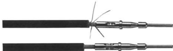
Incorrectly crimped contact
