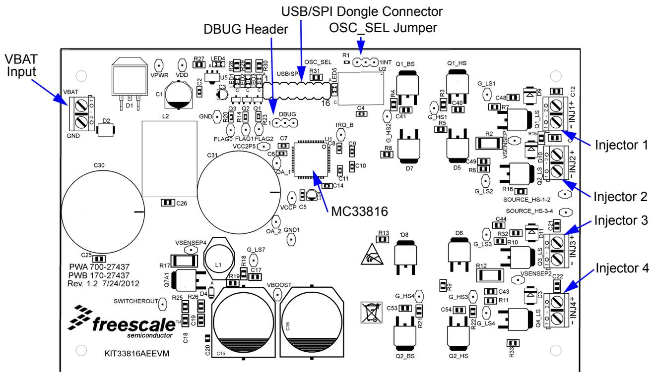
Figure 5. KIT33816AEEVM Evaluation Board Diagram
