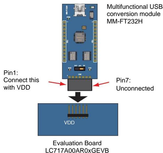
When connecting Multifunctional USB conversion module, make sure to have USB cable unplugged.
