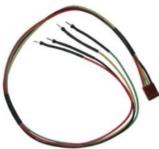
Figure 6: Breadboard Cable (BBC)
