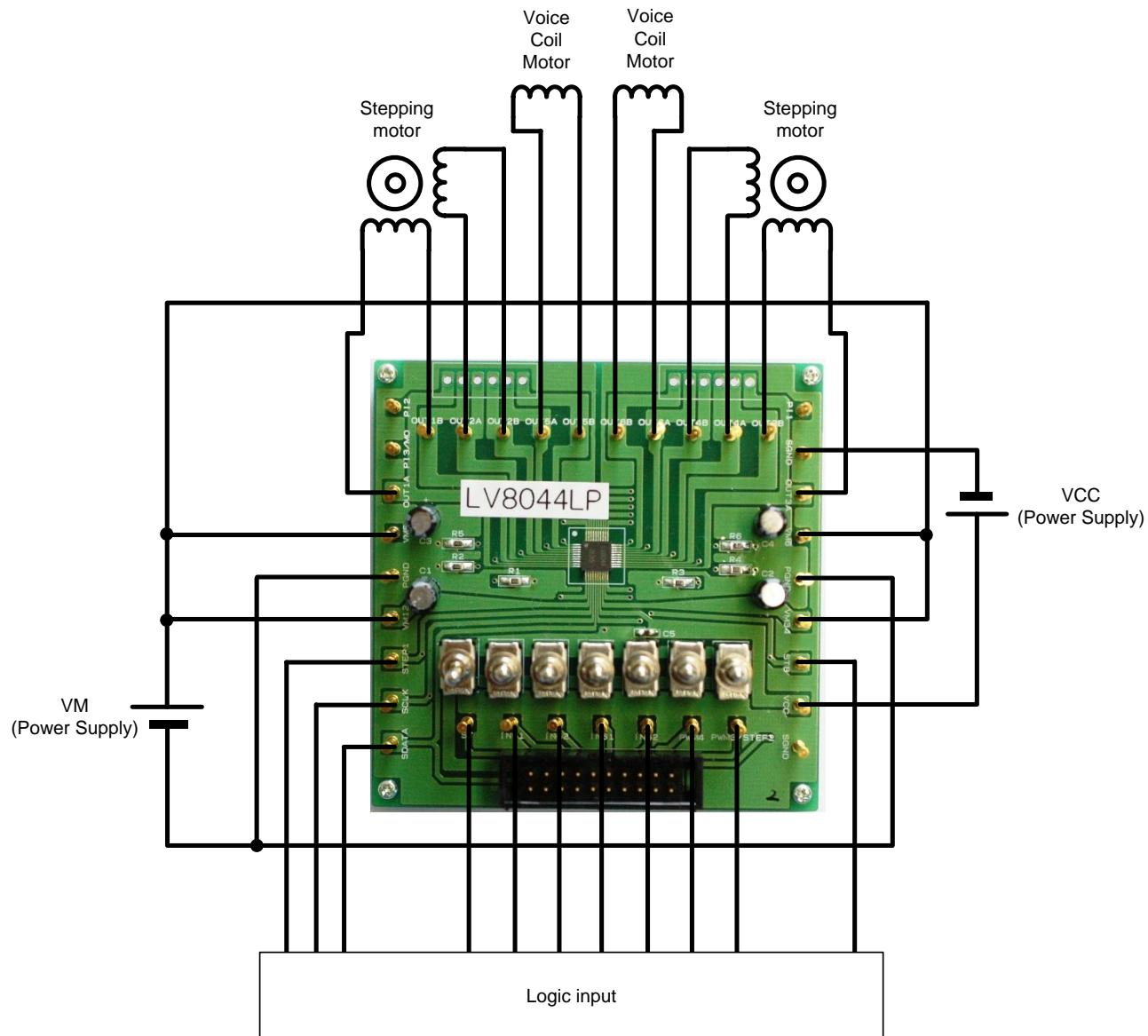
(Circuit diagram of the evaluation board)
