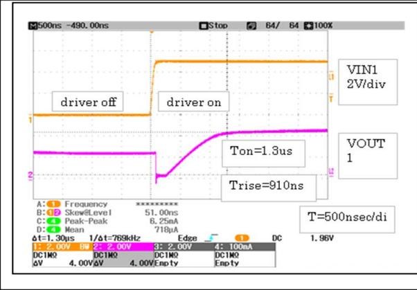
RFG-GND shorted load is 10kohm pullup & down (Fast decay)
