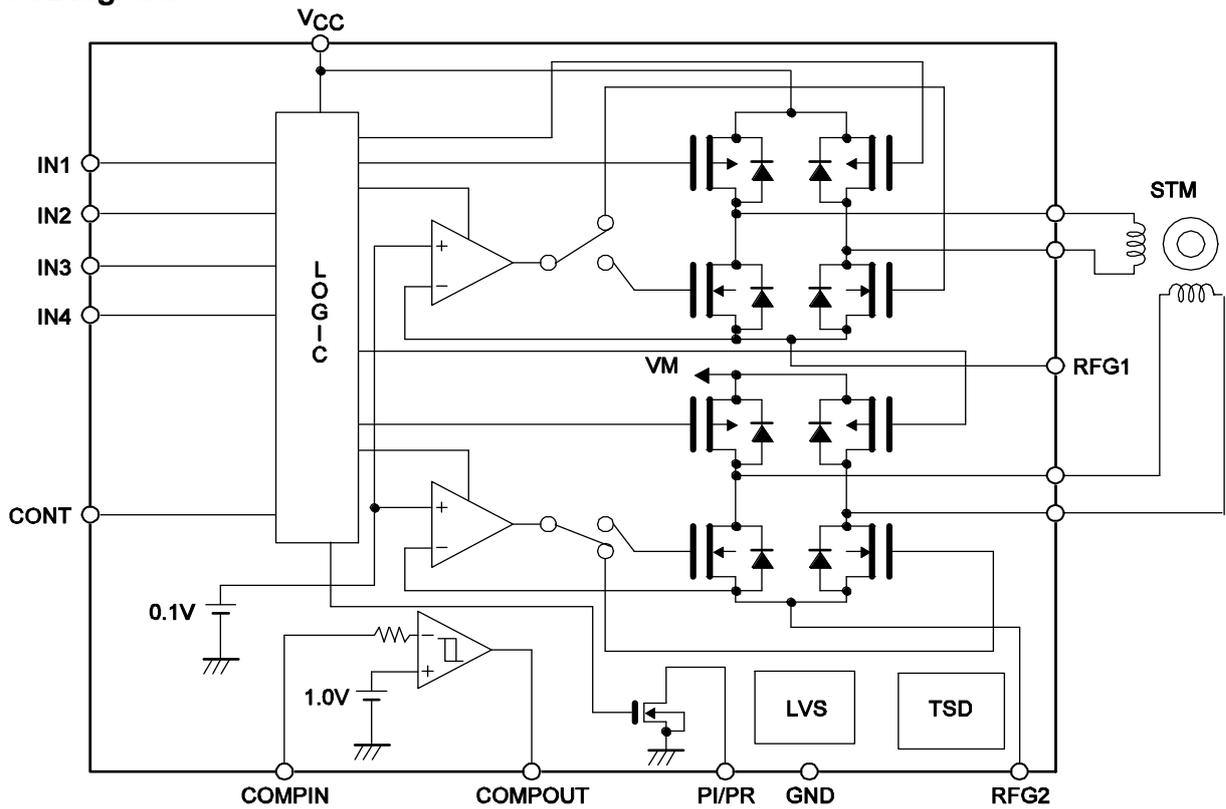
Constant-current calculation :  $I_{OUT} = 0.1 \div R_F$  Example : When an  $I_{OUT}$  of 100mA is required,  $R_F$  must be  $1\Omega$ .
