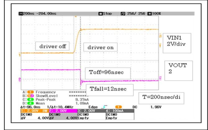
VCC = 3V, VIN1 = 100kHz, 3V, duty50%, VIN2 = 0V input
