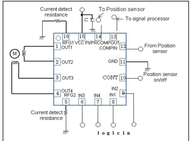
3. Example of applied circuit when connecting in parallel
