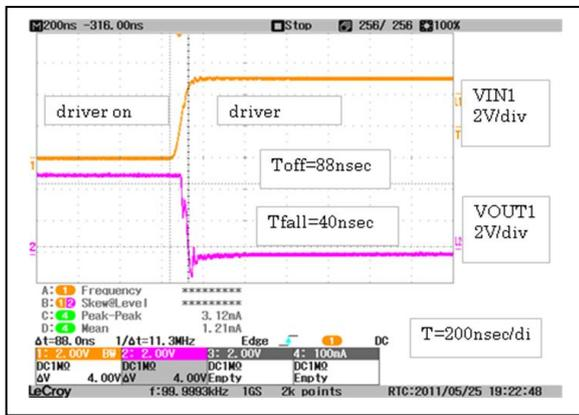
VCC = 3V, VIN1 = 100kHz, 3V, duty50%, VIN2 = 3V input
