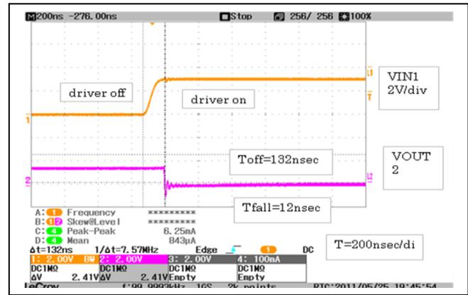
VCC = 5V, VIN1 = 100kHz, 5V, duty50%, VIN2 = 5V input
