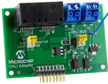
DALI Adapter with 2-wire & RJ45 connections
