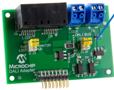
DALI Adapter with 2-wire & RJ45 connections
