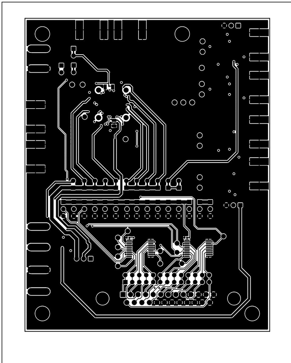
Figure 6. MAX2830 EV Kit PCB Layout—Solder Side
