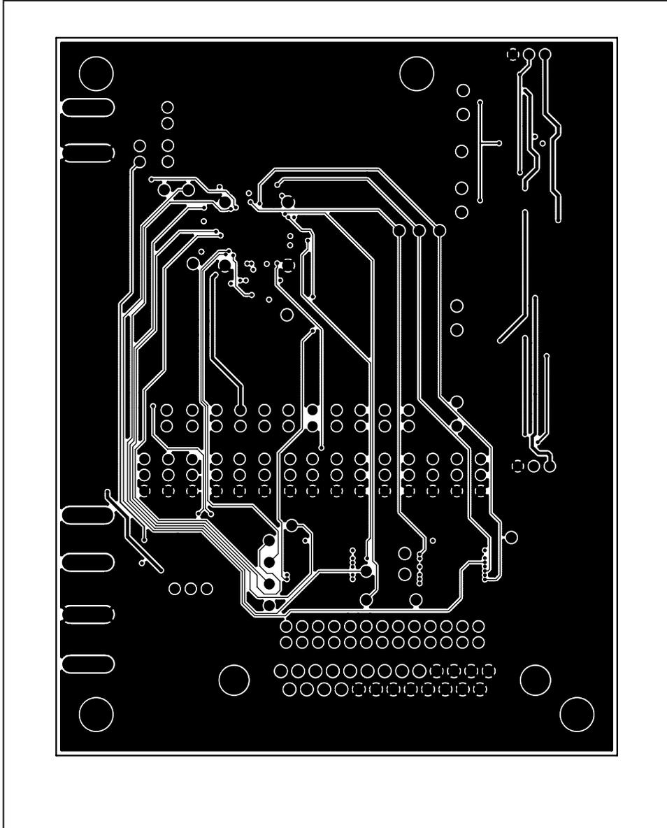
Figure 5. MAX2830 EV Kit PCB Layout—Inner Layer 3 (Routes)
