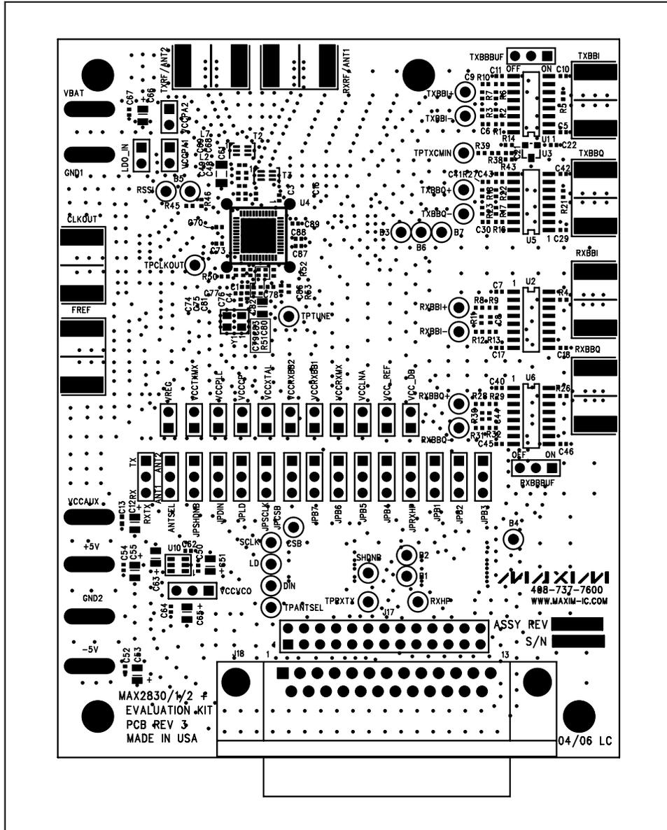
Figure 2. MAX2830 EV Kit PCB Layout—Top Silkscreen
