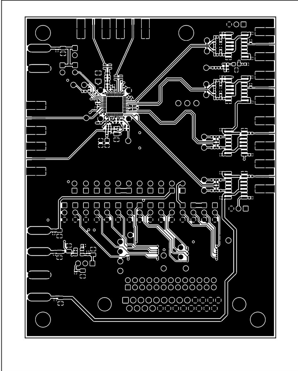
Figure 3. MAX2830 EV Kit PCB Layout—Component Side
