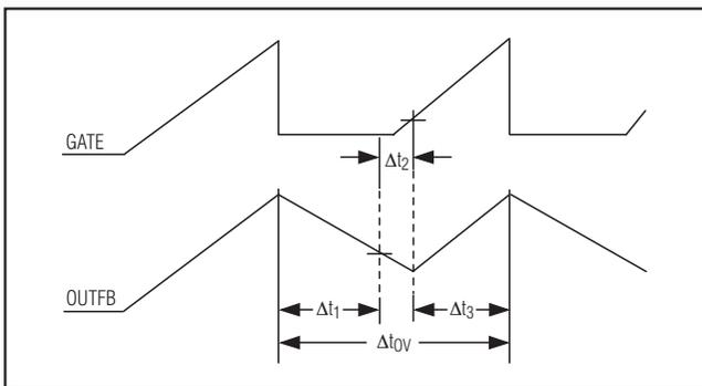
Figure 5. MAX6495/MAX6496/MAX6499 Timing
