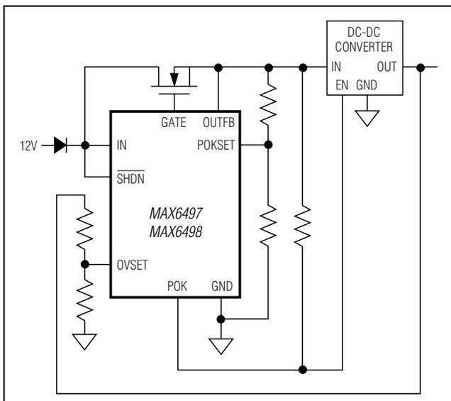
Figure 8. Overvoltage Protection to a DC-DC Converter (MAX6497/MAX6498)
