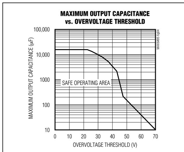
Figure 4. Safe Operating Area for 100mA Pulldown.
