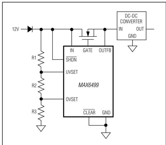
Figure 9. Overvoltage and Undervoltage Window Detector (MAX6499)
