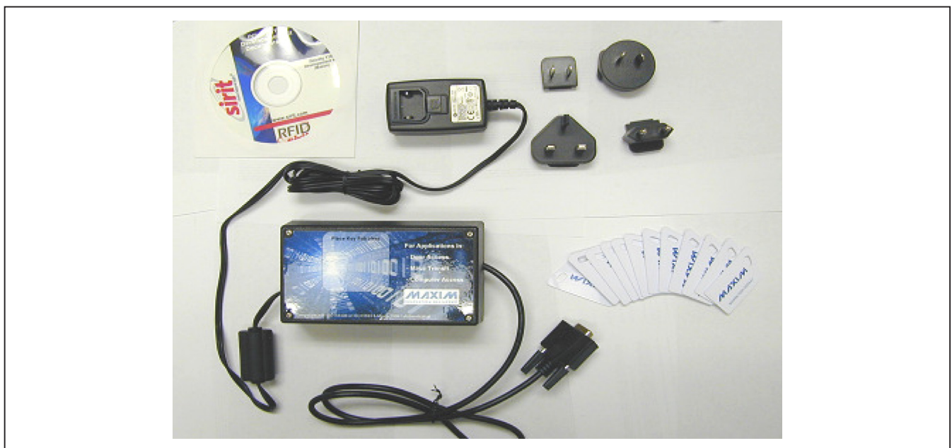
Figure 1. MAX66901 EV Kit Contents
