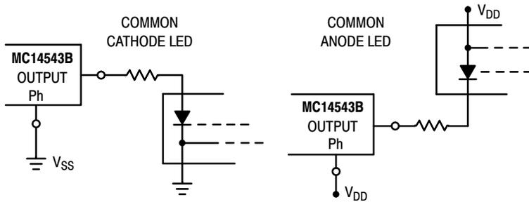
NOTE: Bipolar transistors may be added for gain (for V<sub>DD</sub> ≤ 10 V or I<sub>out</sub> ≥ 10 mA).
