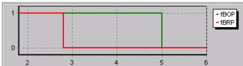
In previous example we see that  $B_{op}$  is programmed around  $5mT$  which means that  $B_{rp}$  is equal to  $(5mT - 2.2mT)$  which is  $2.8mT$  as final  $B_{rp}$ . ( $B_{rp} = B_{op} - hyst$ )
