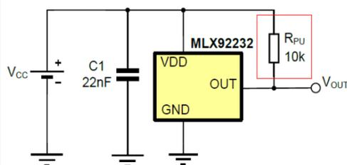
In some cases the pull-up from the PTC04 needs to be used if there no pull-up available on the module that the user is intent to use. (Ref pg 8 MLX92232\_Preliminary\_Datasheet\_rev1.pdf)
