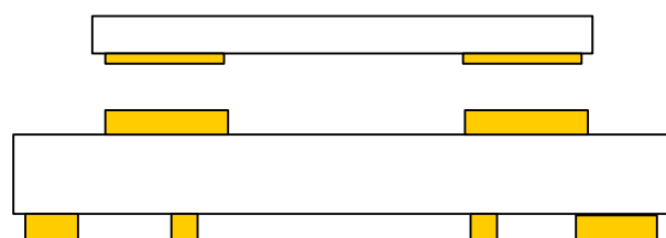
Figure 20. Correct PCB Top Metal Pattern Under Package
