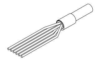
INSERT CABLE, WITH FERRULE, INTO CRIMPING HAND TOOL, WITH APPROPRIATE CRIMP INSERT. CRIMP FERRULE AND TRIM EXCESS SHIELDING AND DRAIN WIRE
