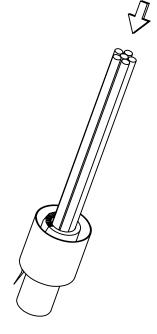
BEFORE CRIMPING FERRULE, IT IS RECOMMENDED, THAT OPERATOR PRE-ARRANGE CONDUCTORS INTO APPROPRIATE TERMINATION SEQUENCE, FOR EASIER POST-CRIMPING ARRANGEMENT.
