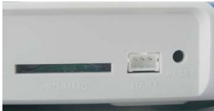
Figure 4. UART Port and SD/MMC Slot on MPC8308-NSG
