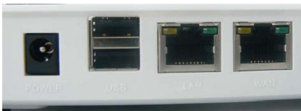
Figure 3. Ethernet and USB Ports on MPC8308-NSG
