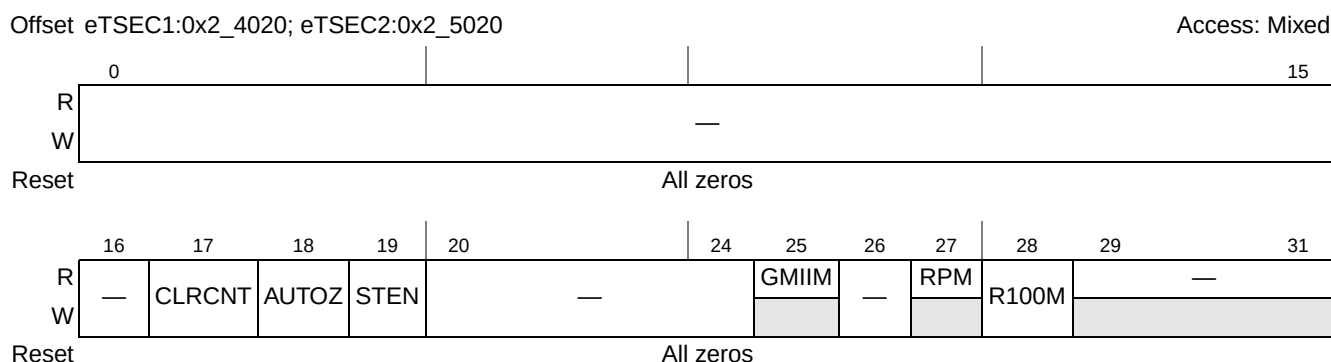
Figure 16-7. ECNTRL Register Definition
