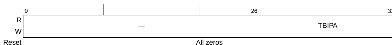
Figure 16-10. TBIPA Register Definition
