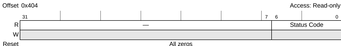
Figure 14-77. PCI Express LTSSM State Status Register (PEX_LTSSM_STAT)
