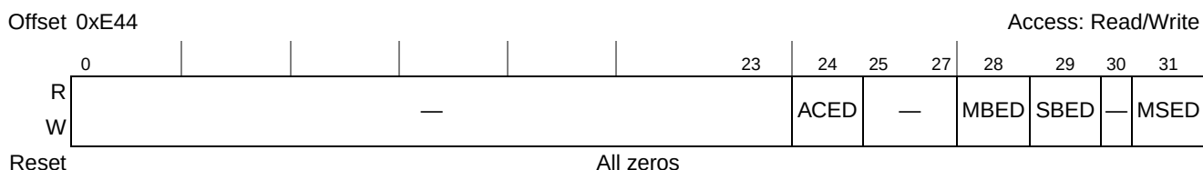
Figure 9-26. Memory Error Disable Register (ERR_DISABLE)
