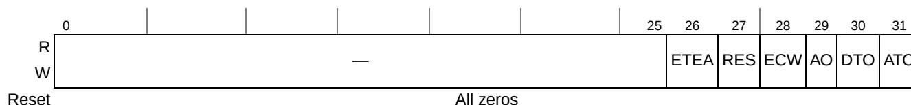
Figure 6-6. Arbiter Mask Register (AMR)
