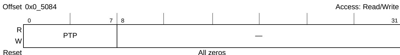
Figure 10-8. Memory Refresh Timer Prescaler Register (MRTPR)
