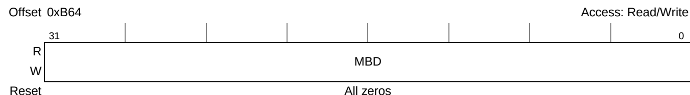
Figure 14-111. PCI Express Inbound Mailbox Data Register (PEX_IMBDR)
