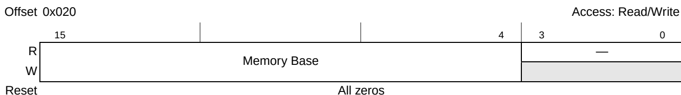
Figure 14-29. PCI Express Memory Base Register
