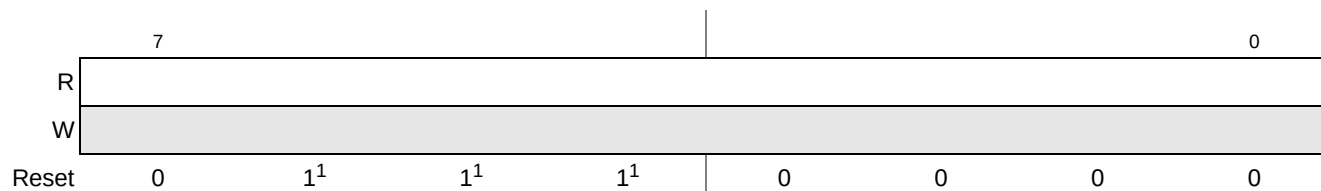
Figure 14-47. PCI Express Next Capabilities Pointer
