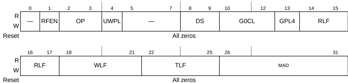
Figure 10-7. UPM Mode Registers (MxMR)
