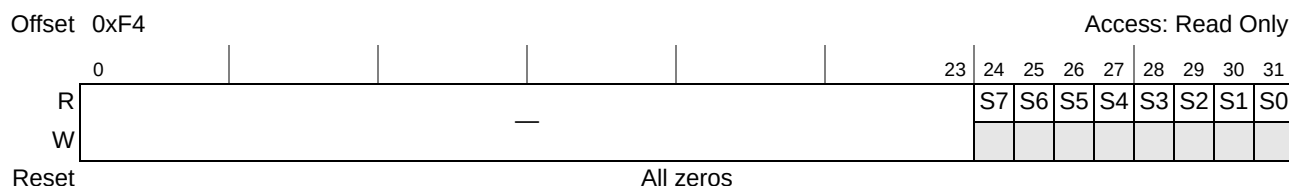
Figure 8-32. Message Shared Interrupt Status Register (MSISR)
