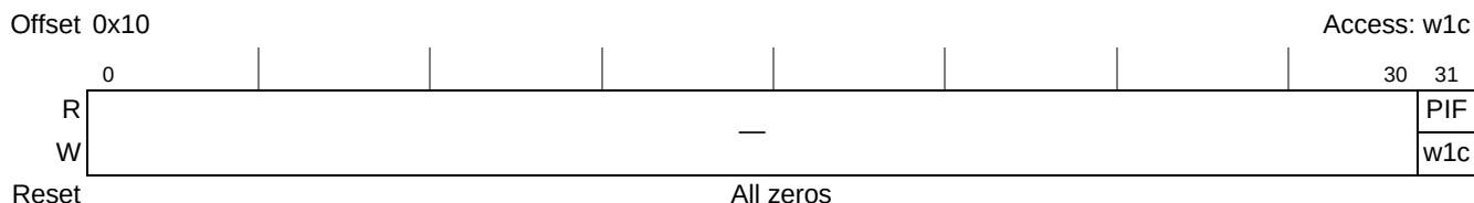
Figure 5-40. Periodic Interval Timer Event Register (PTEVR)
