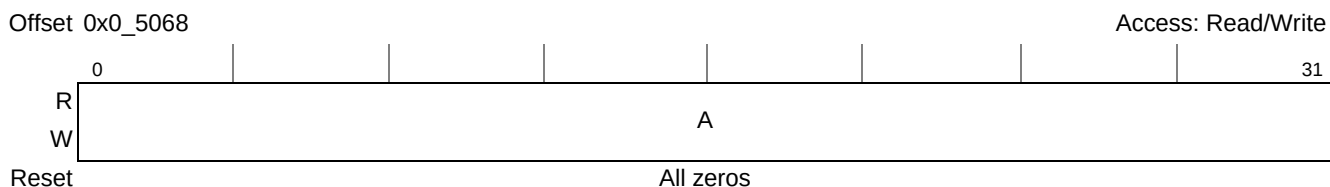
Figure 10-6. UPM Memory Address Register (MAR)
