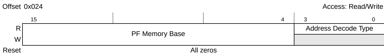
Figure 14-31. PCI Express Prefetchable Memory Base Register
