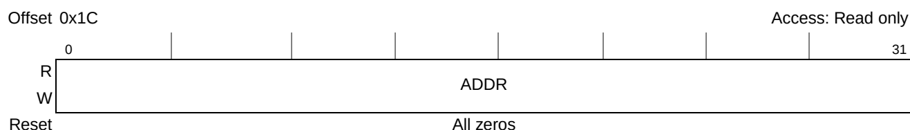
Figure 6-8. Arbiter Event Address Register (AEADR)
