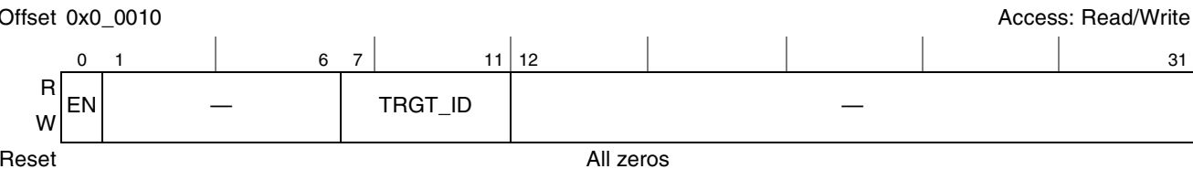
Figure 4-3. Alternate Configuration Attribute Register (ALTCAR)
