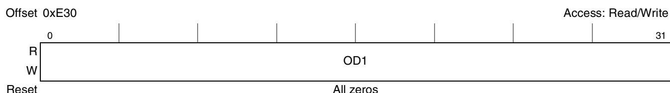
Figure 17-32. PCI Express Error Capture Register 2 (PEX_ERR_CAP_R2) Internal Source, Outbound Transaction
