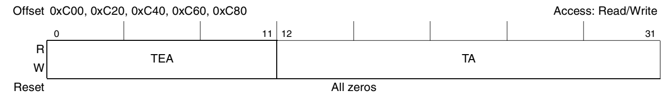
Figure 16-6. PCI Outbound Translation Address Registers (POTARn)
