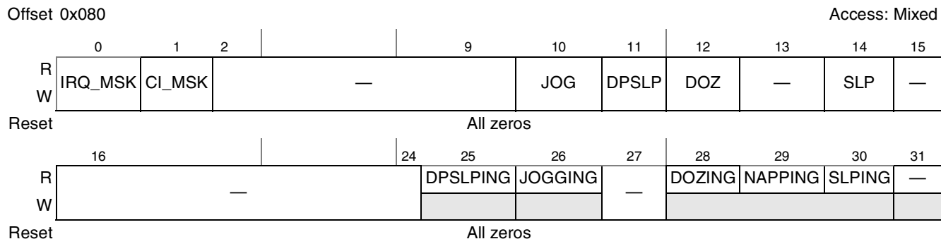
Figure 23-12. Power Management Control and Status Register (POWMGTCSR)
