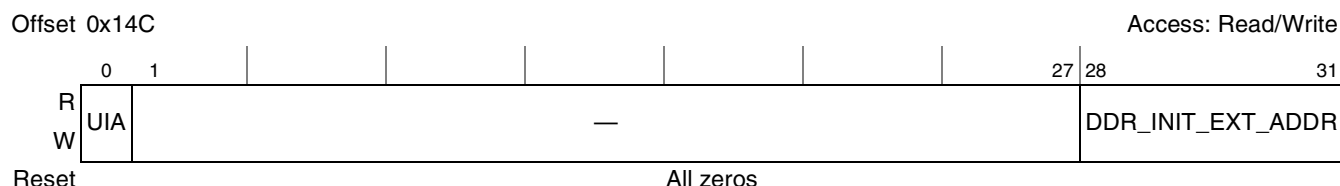
Figure 8-18. DDR Initialization Extended Address Configuration Register (DDR_INIT_EXT_ADDR)
