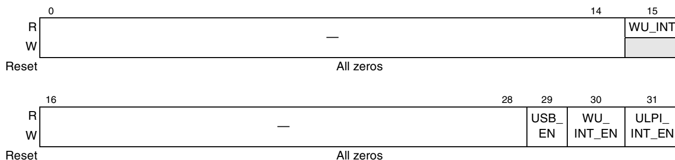
Figure 21-33. USB General-Purpose Register (CONTROL)
