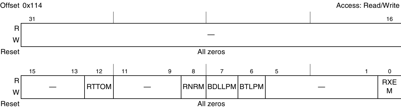
Figure 17-107. PCI Express Correctable Error Mask Register
