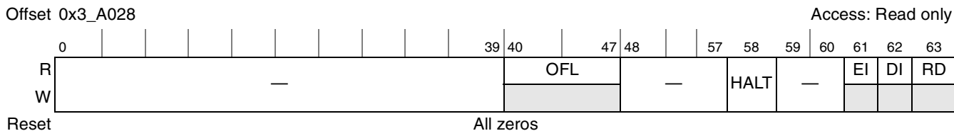
Figure 10-106. RNGU Status Register
