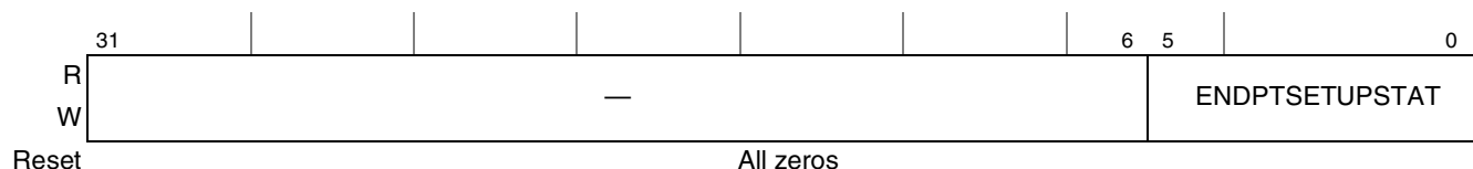
Figure 21-22. Endpoint Setup Status (ENDPTSETUPSTAT)
