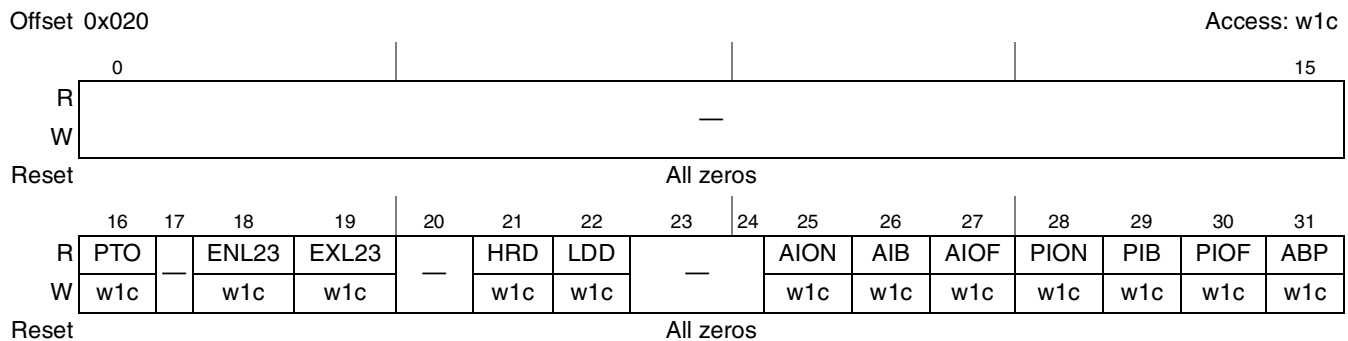
Figure 17-7. PCI Express PME and Message Detect Register (PEX_PME_MES_DR)
