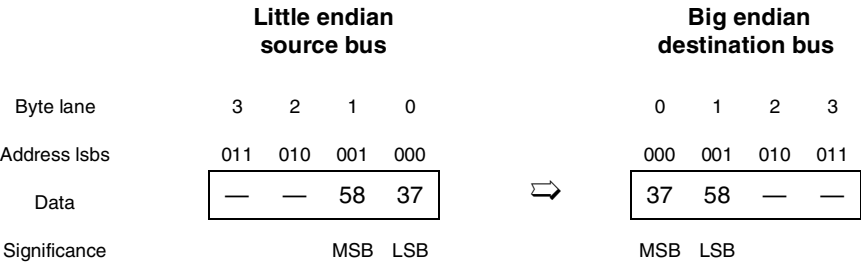
Figure 16-64. Address Invariant Byte Ordering—2 bytes Inbound
