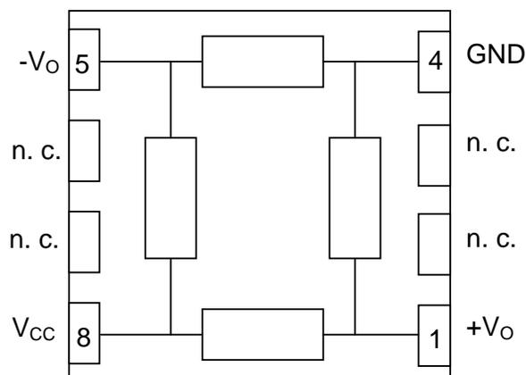
Figure 1: internal and external connections (TDFN, Chip)
