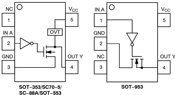
Figure 1. Pinout
