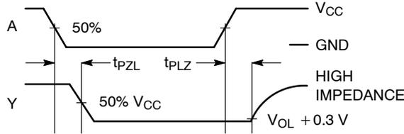
Figure 3. Switching Waveforms
