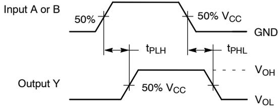
**Figure 3. Switching Waveforms**
