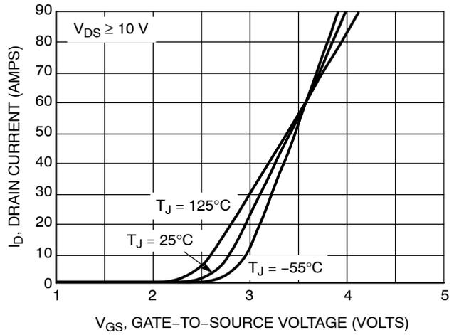
Figure 2. Transfer Characteristics
