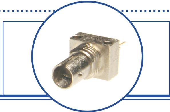
The OPF372 family fiber optic transmitters are high performance devices packaged for data communication links. This transmitter is an 850nm GaAlAs LED and is specifically designed to efficiently launch optical power into fibers ranging in size from 50/125 $\mu$ m up to 200/300 $\mu$ m diameter fiber. Multiple power ranges with upper and lower limits are offered which allows the designer to select a device best suited for the application.
