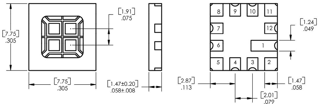
TOLERANCE IS  $\pm .005$  [0.13] DIMENSIONS ARE IN INCHES AND [MILLIMETERS].
