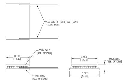
Solder Construction: 138°C, Bismuth Tin Tlam Substrates
