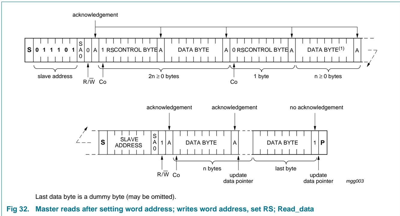
Fig 32. Master reads after setting word address; writes word address, set RS; Read\_data
