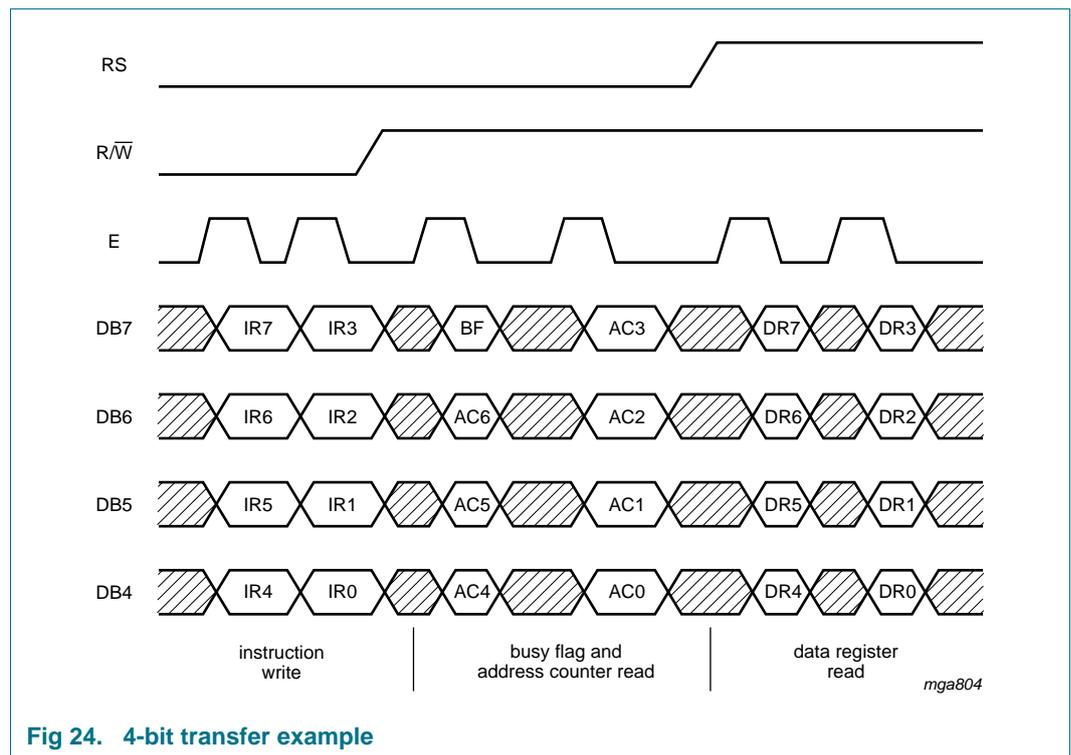
Fig 24. 4-bit transfer example
