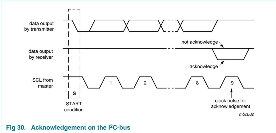
Fig 30. Acknowledgement on the I<sup>2</sup>C-bus
