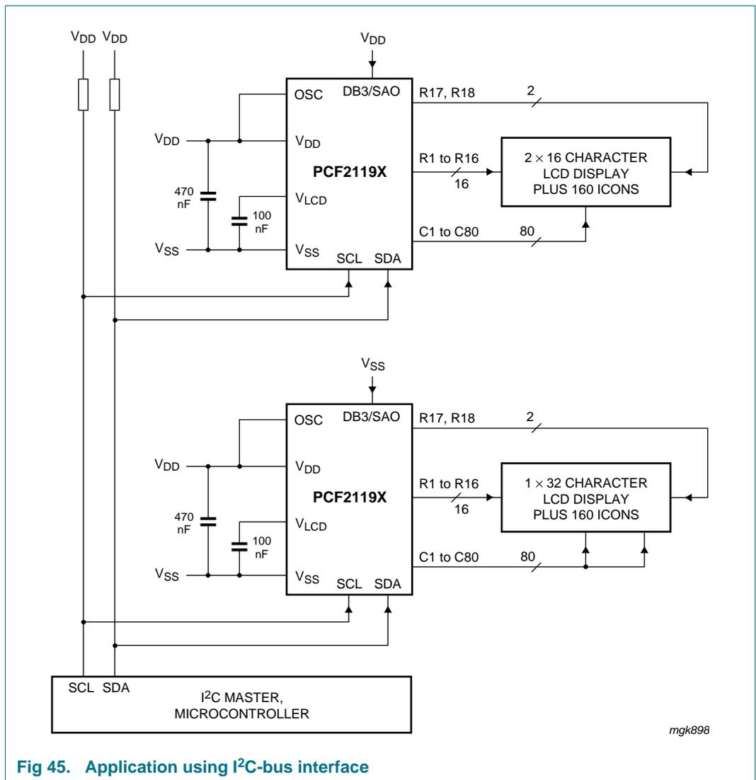
Fig 45. Application using I<sup>2</sup>C-bus interface
