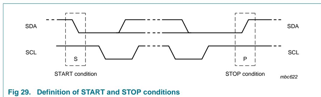
Fig 29. Definition of START and STOP conditions
