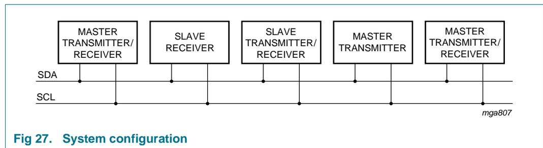
Fig 27. System configuration
