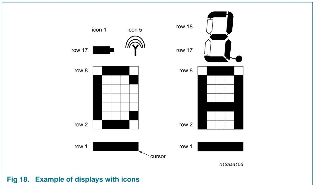
Fig 18. Example of displays with icons
