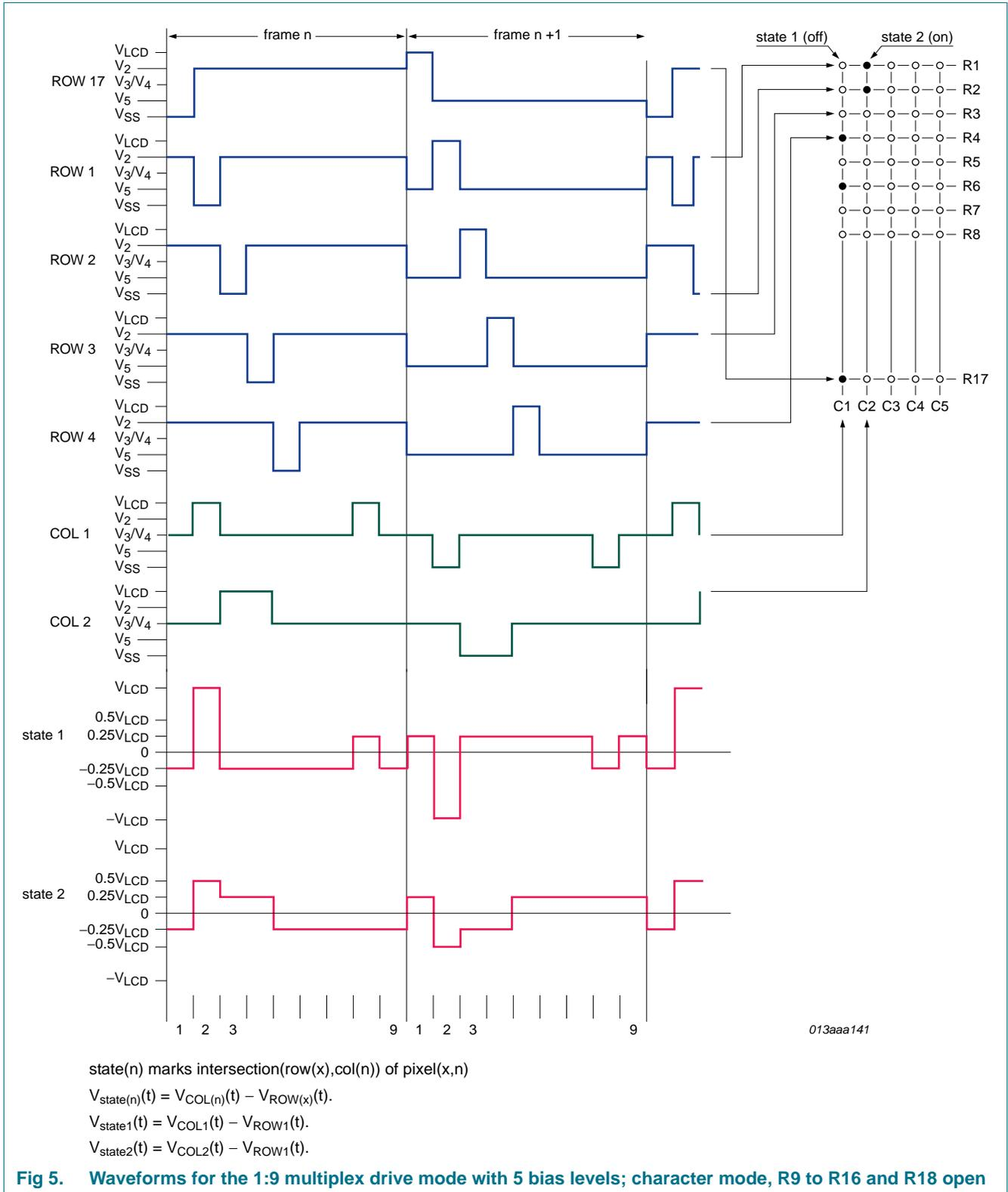
Fig 5. Waveforms for the 1:9 multiplex drive mode with 5 bias levels; character mode, R9 to R16 and R18 open
