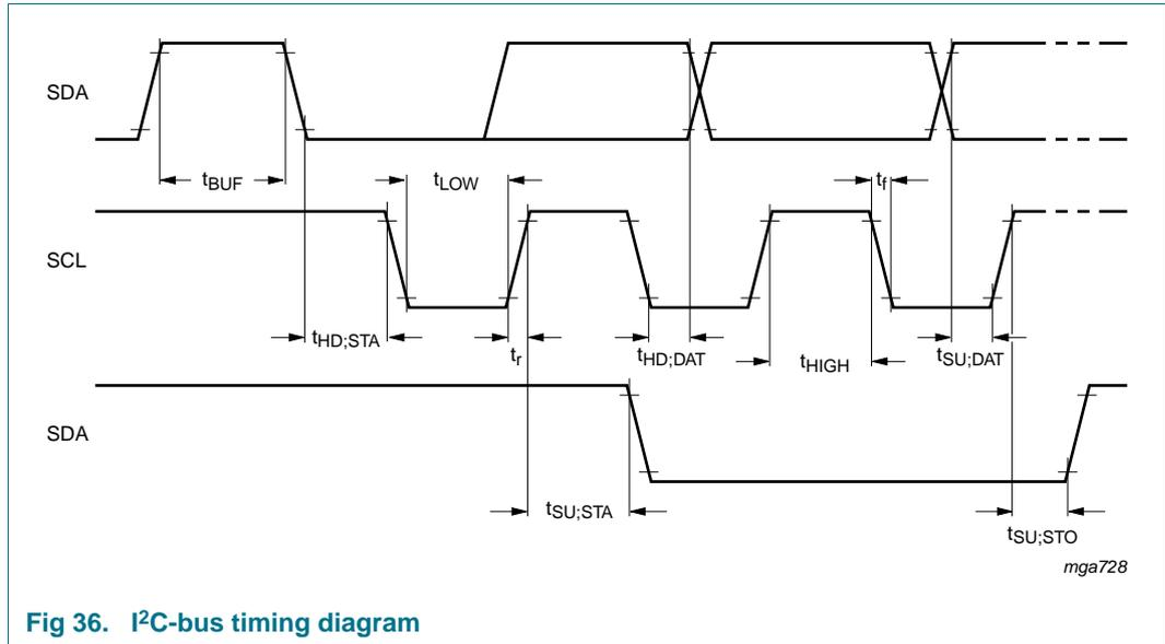
Fig 36. I<sup>2</sup>C-bus timing diagram
