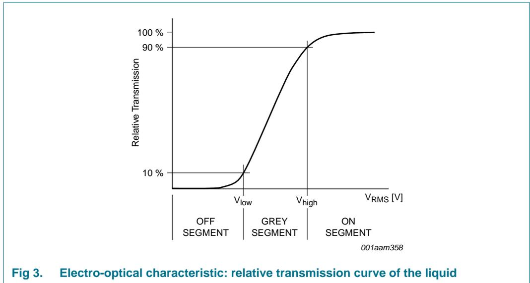
**Fig 3. Electro-optical characteristic: relative transmission curve of the liquid**
