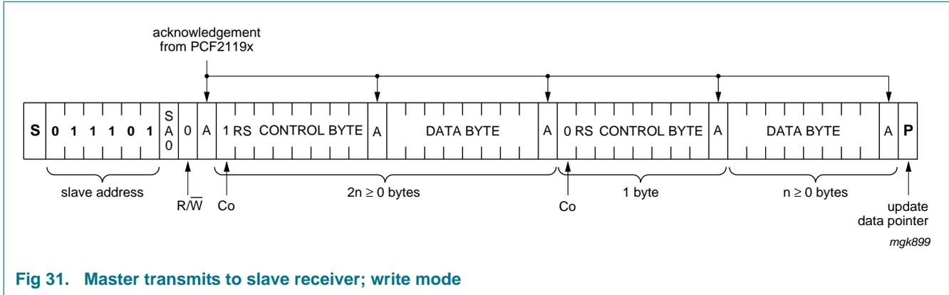
Fig 31. Master transmits to slave receiver; write mode
