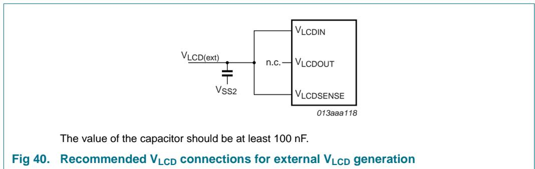
**Remark:** When using an external  $V_{LCD}$ , the internal  $V_{LCD}$  generator **must never** be switched on and direct mode must be avoided otherwise damages will occur.
