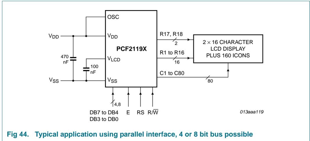
Fig 44. Typical application using parallel interface, 4 or 8 bit bus possible
