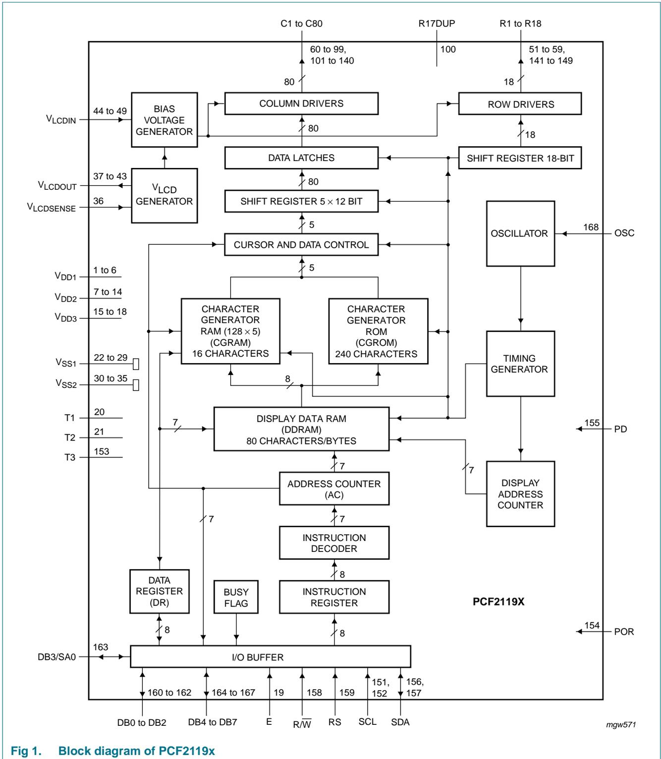
Fig 1. Block diagram of PCF2119x
