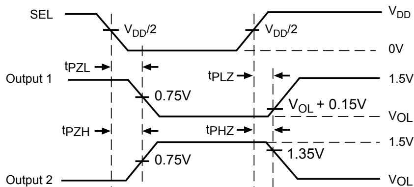
**Voltage Waveforms Enable and Disable Times**
