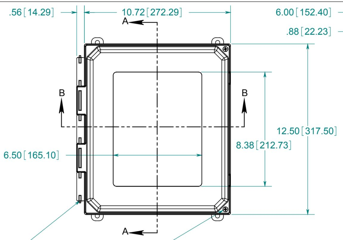
STAINLESS STEEL HINGE PIN AND (2) STAINLESS STEEL PUSH NUT FASTENERS
