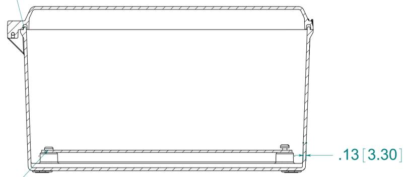
(4) EACH #10-32 BRASS INSERTS AND PLATED CARBON STEEL SCREWS
