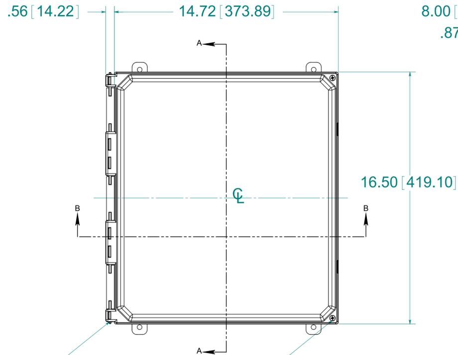
STAINLESS STEEL HINGE PIN AND (2) STAINLESS STEEL PUSH NUT FASTENERS
