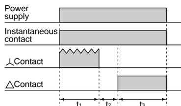
$t_1$ : ∩ operation time (∩ indicator LED lights)
