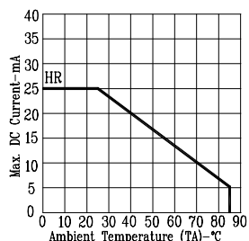
Fig5. MAX. ALLOWABLE DC CURRENT VS. AMBIENT TEMPERATURE.
