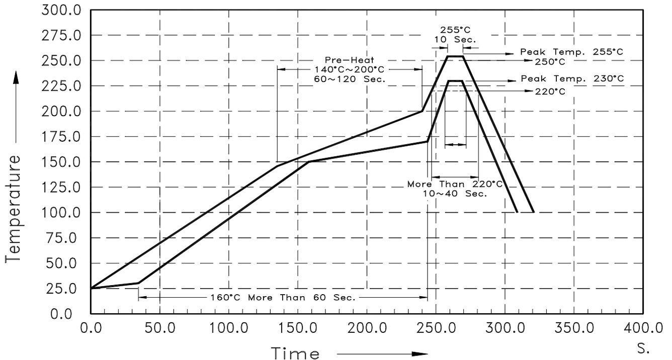
The Profile is available that must to use SnAg (x=3.3~3.8) Cu (y=0.2~0.7) solder paste
