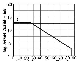
Fig5. MAX. AVERAGE FORWARD CURRENT VS. AMBIENT TEMPERATURE.
