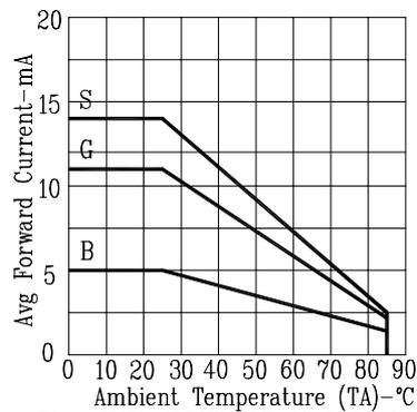
Fig. 4. MAX. ALLOWABLE DC CURRENT VS. AMBIENT TEMPERATURE.
