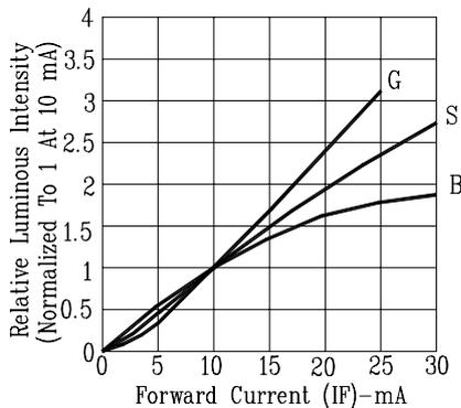
Fig. 3. RELATIVE LUMINOUS INTENSITY VS. FORWARD CURRENT
