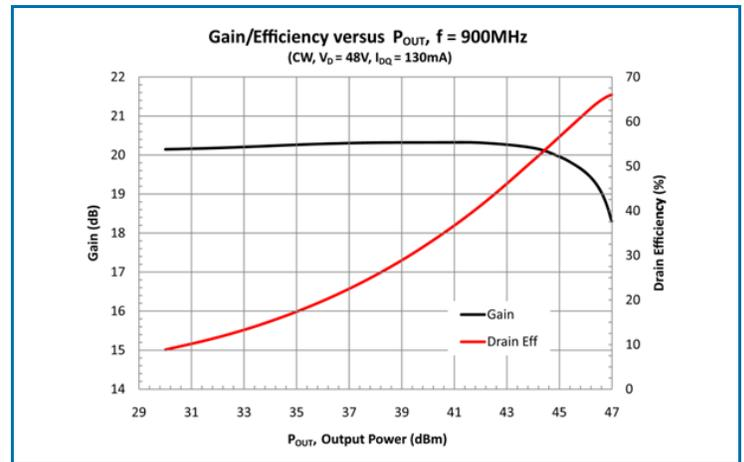
**Typical Performance** in standard 900MHz fixed tuned test fixture
