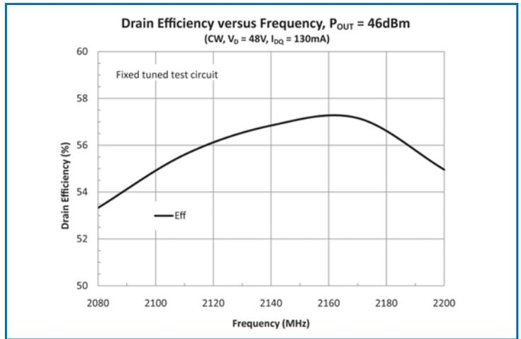
**Typical Performance** in standard 2.14GHz fixed tuned test fixture
