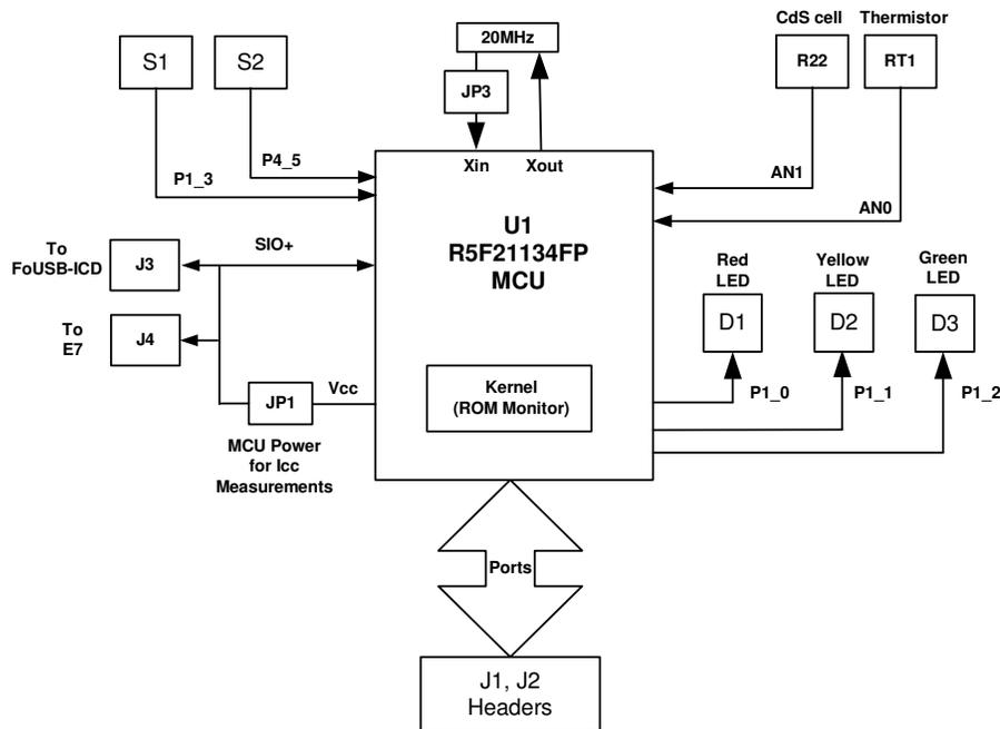
Figure 5-2. Mini R8C Board Block Diagram
